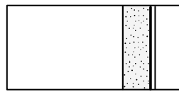
Drywall without available wood stud
